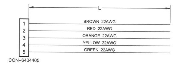
NOTE: FOR CABLES LONGER THAN 4 FT.(48in.), USE CBL-22AWG-8COND-SH.
